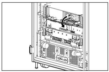
Figure 1-30: Closing the locking handle
